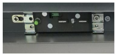
When the correct height has been confirmed by the green catch clicking, the soft close function closes the door correctly with no gaps the activator can be secured to the top track using 2 x 20mm screws.
