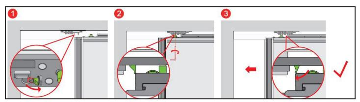
To remove a door, the bottom running wheels will need to be adjusted lower and therefore will disengage the soft close mechanism. Please see the door adjustments in how to raise the door up.
