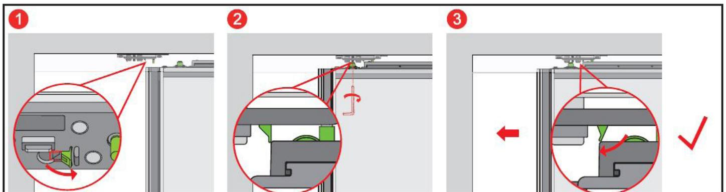
To remove a door, the bottom running wheels will need to be adjusted lower and therefore will disengage the soft close mechanism. Please see the door adjustments in how to raise the door up.
