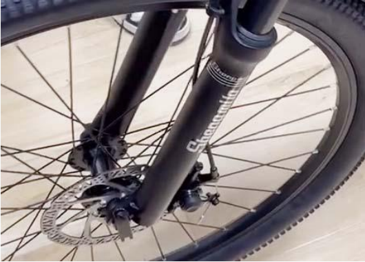
2. Tighten the wing nut to align the quick release lever with the shaft.
