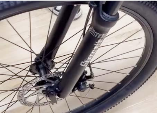
3. Make sure the quick release lever on the front wheel is fully closed.
