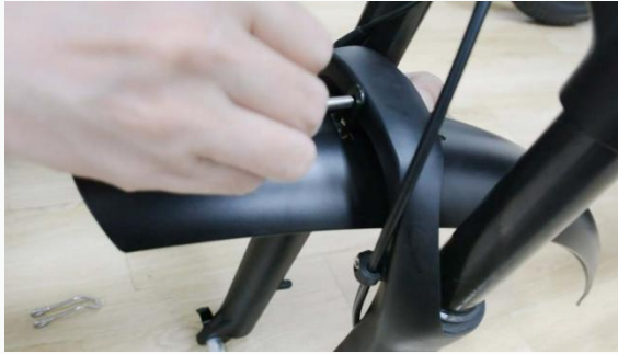
2. Tighten the bolts with 6mm wrench retaining nuts.
