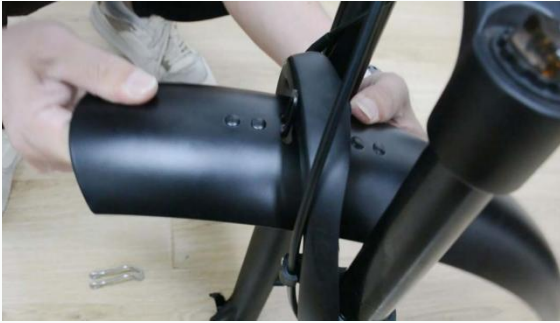
1. Align the front fender bolt holes with the holes in the holder.
