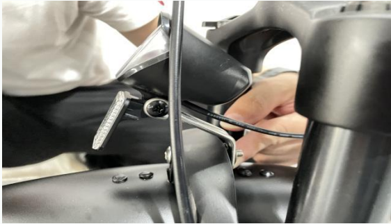
1. Align the headlight bolt holes with the holes on the fork bracket
