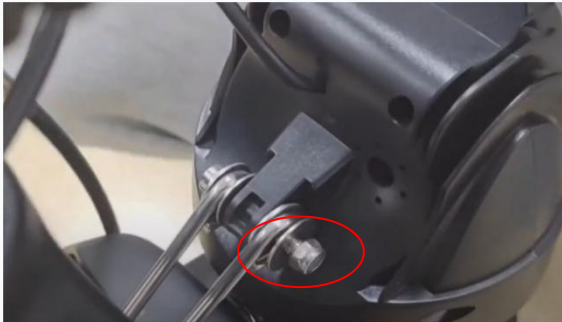
3. Set the nut to tighten the bolt
