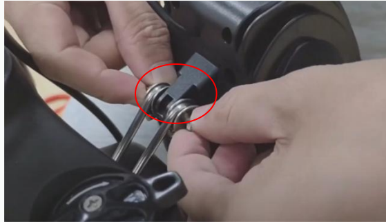
2. Align the headlight bolt holes with the holes on the fork bracket
