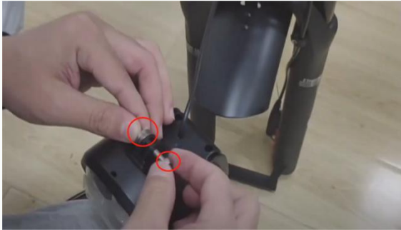
1. Loosen the bolts on the headlights with a PH1 wrench
