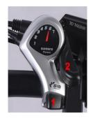
When you are riding on flat ground or road, you can use the button (2) to adjust to your suitable small gear.
