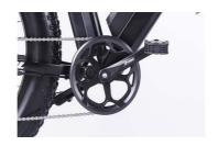
Left pedal (2) tightens counterclockwise
