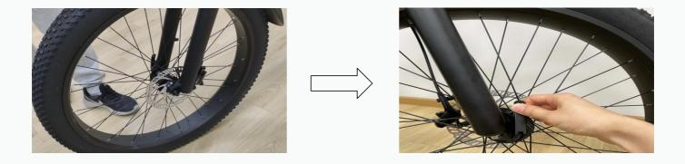
**Step 6:** Rotate the front wheel. Make sure the quick release skewer lever on the front wheel is fully closed, and check the wheel balance in Pedal-Only Mode. If you notice the riding is imbalanced or the rotation of the front wheel makes noise, it means the bolts were not completely tightened or not aligned horizontally.
