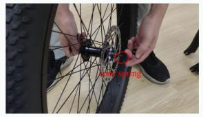
**Step 3:** Tighten the thumb.
