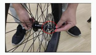
Step 4: Align the fork dropouts with the axle of the wheel hub, making sure the dropouts are securely positioned on the axle. Also ensure the brake rotor is properly inserted into the caliper.
