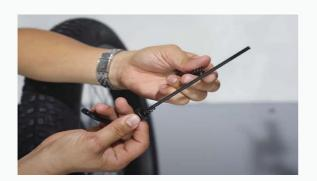
**Step 2:** Install the quick-release skewer starting from the brake rotor side of the wheel, inserting the quick-release skewer through the hub and then replacing the second cone spring on the other side. Ensure both springs are pointed narrow-side-in towards the wheel hub.
