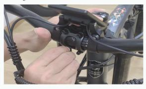
Step 3:: Tighten bolts to handlebar stem, but don't tighten completely as you may want to further adjust the angle later to align more precisely. After determining the best position, completely tighten all the bolts on the stem.
