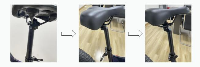
**NOTICE:** The seat angle has been preadjusted to factory safety standards. Please make note of original settings, and only adjust if necessary.
