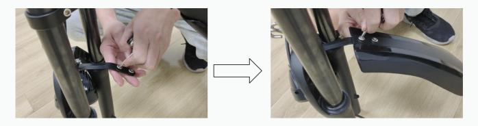
1. Loosen the bolts on the front fender holder with a 6mm hex wrench.
