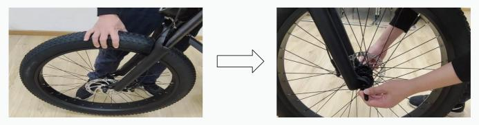
Step 5: Tighten the thumb nut until the quick-release lever is held in line with the axle, and then use your palm of your hand to close the quick-release lever.
