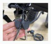
**Step 2:** Use the key to unlock the battery. While holding the battery with one hand, detach the battery by turning the release switch located on the underside of the frame.
