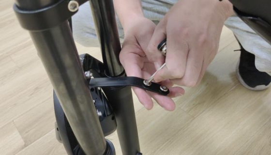
1. Loosen the bolts on the front fender holder with a 6mm hex wrench.
