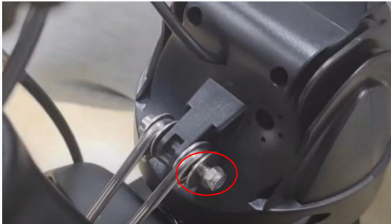
3. Set the nut to tighten the bolt
