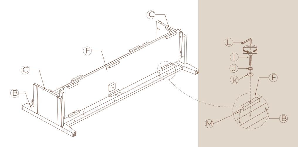
Insert the Divider panel H to Bottom panel F, and Frame B using Wood dowels M, Bolts I, Lock washers J, Flat washers K, and Allen key L. Do not fully tighten yet.
