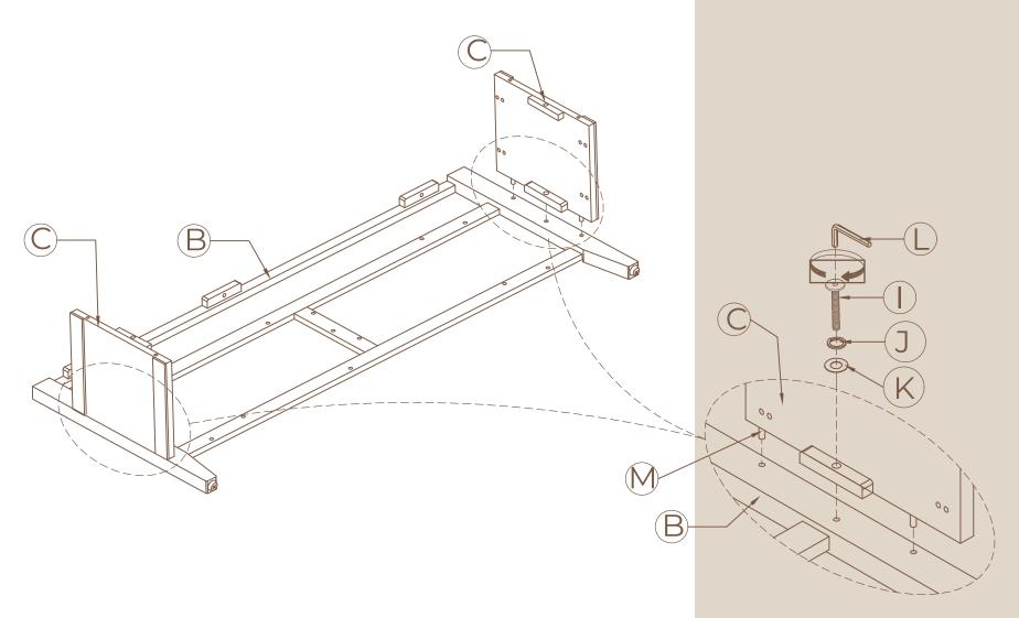
Insert the Bottom panel F to Frame B, and Side panels C using Wood dowels M, Bolts I, Lock washers J, Flat washers K, and Allen key L. Do not fully tighten yet
