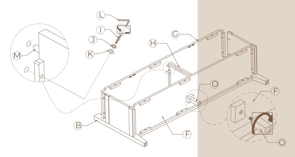
Insert the Back panel E to Side panels C, Divider panel H, Shelf panel G, and Bottom panel E using Wood dowels M, Bolts I, Lock washers J, Flat washers K, and Allen key L. Do not fully tighten yet
