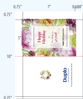
Optional Slitter Cassette: Letter size 1-up 5" x 7" greeting cards with 1 fold
