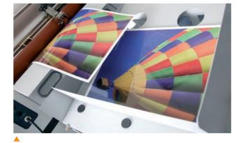
Gloss over guickly, matt in minutes The automatic separator works fluidly with the laminator, ensuring your job is ready for the next stage the moment it's through.
