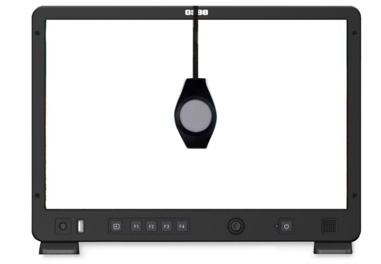
Figure 5.2-29 Calibration Probe on Screen
