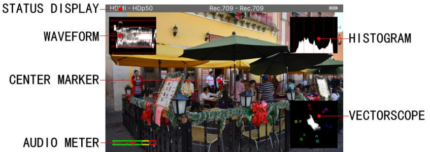
Figure 5-2 Tools for T5+ Monitor
