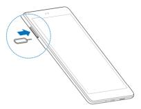
2. Pull out the card tray and place the nano-SIM card and the optional microSDXC card on the tray, as shown. Carefully slide the tray back into place.
