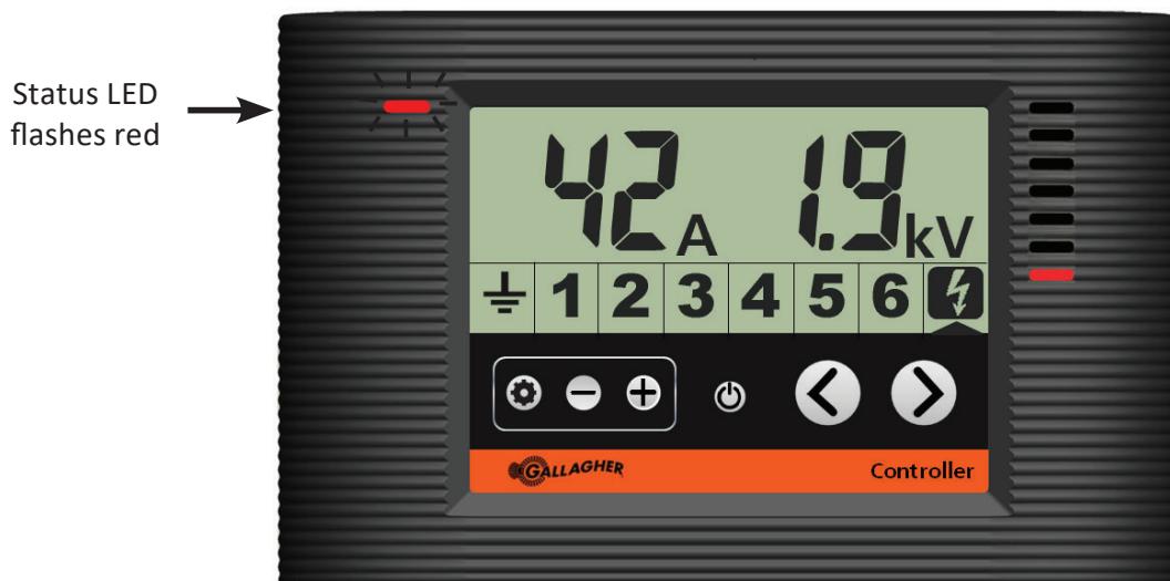
Controller showing the energizer in output alarm
