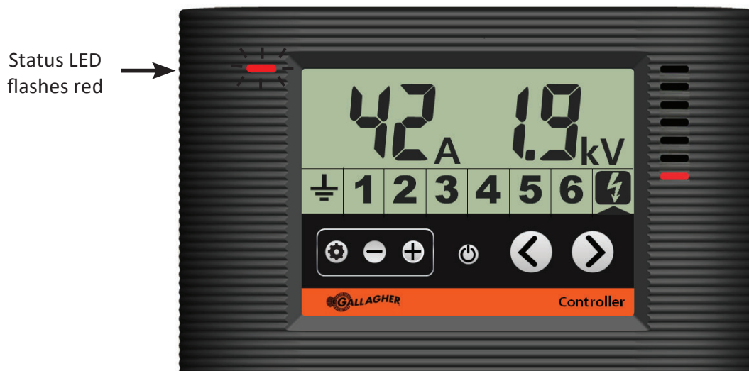
Controller showing the energizer in output alarm
