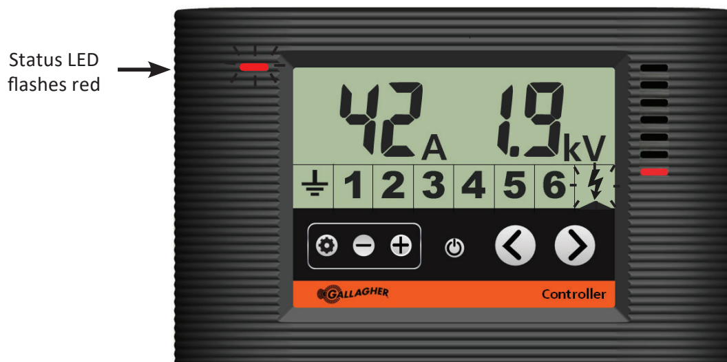
Controller showing the energizer in current alarm
