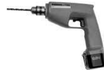
Drill and 3/8" Drill Bit
