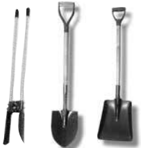
Post Hole Digger - hand held Shovels - spade type and regular
