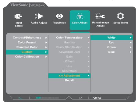
**5.** Touch the **1** or **2** key to select the x or y coordinate and touch the **3** key. Then touch the **1** or **2** key to adjust the setting.
