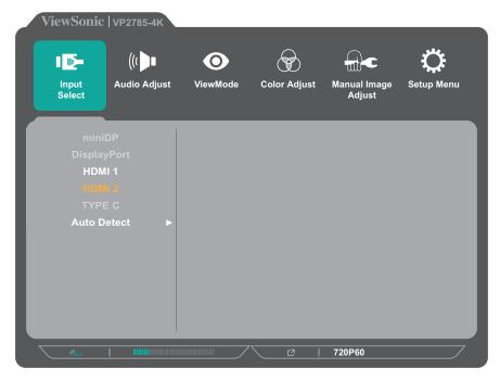
**3.** Touch the **1** or **2** key to select the desired input source. Then touch the **3** key to confirm the selection.
