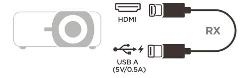
1. Connect the Receiver's HDMI Output to an **HDMI** port of the projector.
