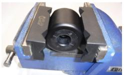
• Slide the socket clamp guide and socket assembly into the jig holder with the tapered end of the clamp guides facing out.
