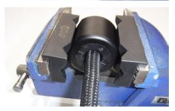
• Using a twisting and pushing motion, push the hose into the clamp guide and jig holder until the hose seats firmly in the hose end.
