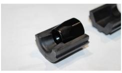
Place your hose end socket into the socket clamp guide with the narrow end of the socket toward the tapered end of the socket clamp guide.
