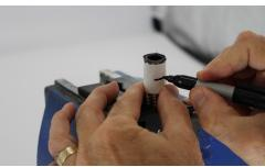
• Using a low residue tape wrap the area of the hose that you want to cut and then mark your cut length on the tape.
