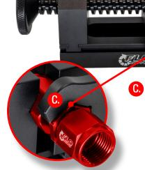
When tightening the B-nut to the hose socket nut, make sure the socket nut is secure within the vise clamps. Choose the correct AN size wrench and tighten the center nut between the hose socket and the B-nut as shown in the photo to the left
