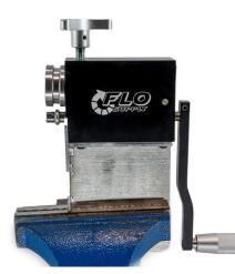
• Clamp tubing bender firmly in a table vise so that the handle operates freely.
