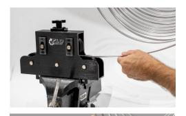
• Without bending the end of the tube too sharply (avoiding kinks) begin to feed the tube through the rollers.
