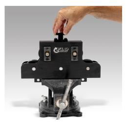
• Loosen the top adjustment knob to allow the open end of your tubing to go through the rollers.
