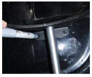
**Step 11:** Mark the loction on the car panel.
