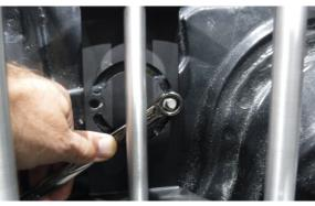
Step 12: Remove the bottle from the mounting bracket, then fasten the bracket in place.
