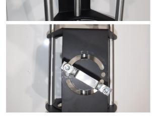
**Angled Bar** – Using a 1/4" Allen wrench and 1/2" wrench, install the roll bar mounts to the top and bottom curved slots on the main bottle bracket.
