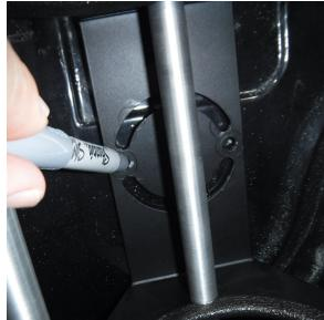
Step 10: Mark the loction on the car panel.
