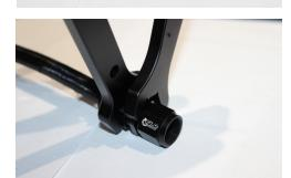
• Now tighten the two sides together until the resistance increases and there are no visible threads between the end and the socket. (the use of Flo Supply AN wrenches helps with this process)
