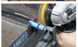
• Using a low residue tape wrap the area of the hose that you want to cut and then mark your cut length on the tape.
