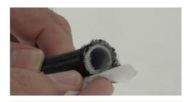
• Clean any dust or material from the hose before moving to the next step. Alcohol or other cleaners may be used but make sure to avoid damaging the PTFE liner or the nylon hose wrap.
