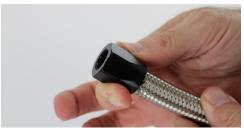
• Insert the hose straight into the hose end socket without fraying the outer hose material. You must screw the hose into the socket in a clockwise rotation.
