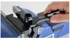
Once you are sure that the hose is not being pushed out of the hose end, use the correct AN
