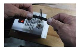
• Cut all sections of sleeving with a hot knife. This will melt the fibers of the sleeving together so that is does not unravel while installing it on the harness.
