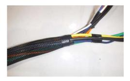
• Using electrical tape, tightly anchor each end using no more than 1 ½ rounds.
