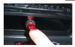
• Once the installation steps have been completed, test the harness for functionality. Flip the switch to the on position, the pump should begin to circulate water. Check for leaks.
