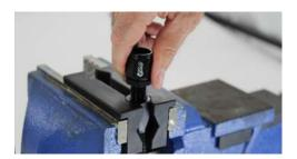
• Carefully center the insert and begin to thread it in the sleeve. It may require a little force to push the fitting nipple into the hose far enough for the threads to engage.
