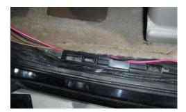
• When routing the individual wires in each section to its connection point and secure them in place. Looming the wires and terminating will be done once routing and length is determined.
