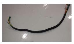
• Feed the section of sleeving from the component end of the harness toward the relay. The best procedure for this is to feed all the sleeving onto the end of the harness. It will look like a compressed spring on the harness.
