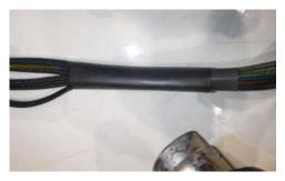
• Using heat shrink, cover the breakout or the branch off to ensure you have no exposed wires. This length will need to cover the end of the sleeving on the first section of wires to the start of the sleeving on the next section of the harness.
