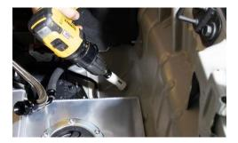
• In the event that the harness needs to route through a drilled hole in the firewall use the supplied grommet to protect the wires from being damaged.
