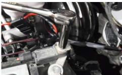
Connect the black 12ga wire leading out of the relay to the negative battery terminal or a known good ground.
