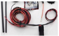
• The main Red 12 gauge wires (2x) will go from the battery to the relay and then from the relay to the pump. This will also include the in-line fuse between the battery and relay. The pump's 12 gauge black wire needs to be sent back to the negative battery terminal or a known good ground.
