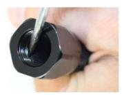
• Make sure the hose liner is flush with the inside of the Cutter Hose end.
