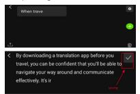
(2)After saving, you can choose to upload to you PC. Click here "upload sign", and connect the translator with you computer through USB cable, you can find the saving text on "Excerpt File"
