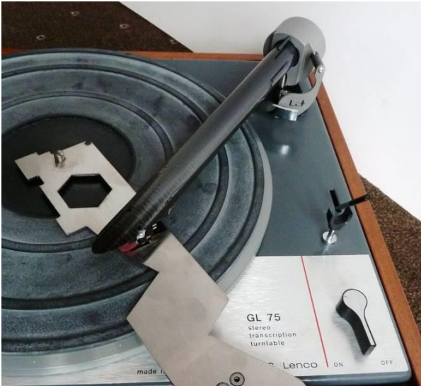
6; Check overhang via protractor, may have to loosen screw and move mounting slightly.
