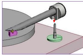
**Step 2;** Ensure the two clamping screws are loosened slightly (1/4 turn anticlockwise)
