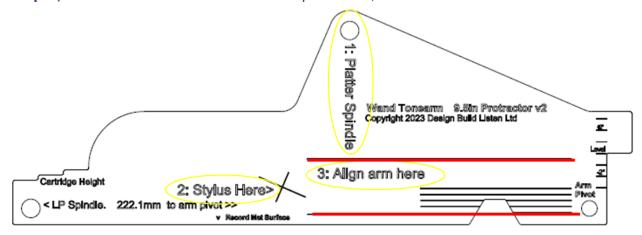
**Step 4**; Then look down from above at the sides of the tonearm and note how they align with the red lines above.
