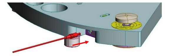
**Step 7;** Lower the platter gently over the spindle. Add the small black mat in the middle. The platter should spin easily. *If it doesn't*, *lift off the platter / spindle and check there is a chrome ball in the bottom of the well (a spare is also supplied). This is hard to see but a cotton bud helps by moving it around.*
