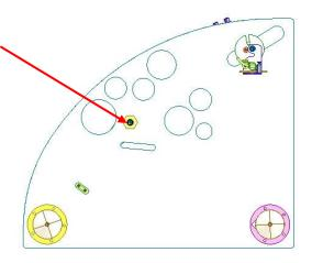
**Step 6**; Plug the wire from the power supply into the socket on the side of the turntable. (But don't plug into the mains power yet)
