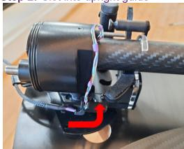
**Step 3**: Slip the braid into the rear clip (or clamp)
