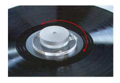
**Step 3**; If you chose, screw the record clamp down clockwise to flatten warped records. Note; It will depend on the record if this helps. You will get fine results without it on most records.
