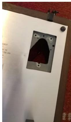
**Hint;** Improve your Thorens by adding damping material to the underside of the sheetmetal panels and the bottom cover while it is off. (but watch adding too much weight to the floating chassis part)
