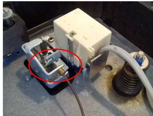
**Step 5;** Remove the cable base (Two screws)
