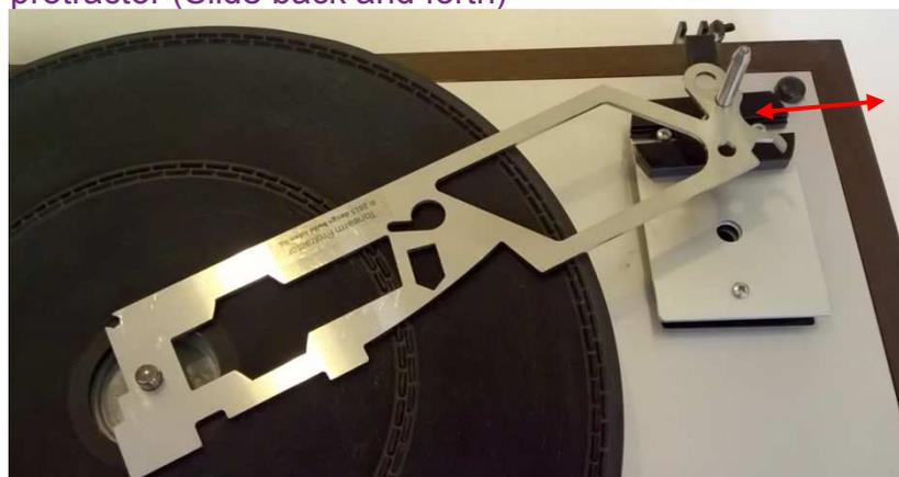
**Step 3; Tighten the three screws**
