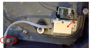
**Step 2**; Support the turntable upside down and remove the bottom cover. 4 screws.
