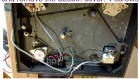
Step 4; Unhook the lift mechanism
