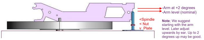
**Step 2**; Position the mount using the protractor (Slide back and forth)
