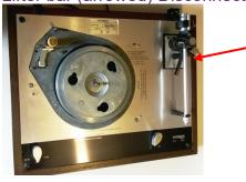
Step 3; Remove the arm cable clamp and the white cable cover.
