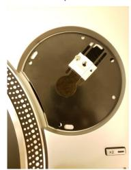
**Step 6**; Set arm height. Do this before bolting plate down (easier access to set height).
