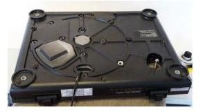
**Step 3**; Detach the earth tag from chassis. (Note this, (green) for attaching earth later)
