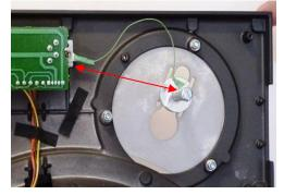
**Step 7;** Position the spindle sideways using protractor (& tighten screws)
