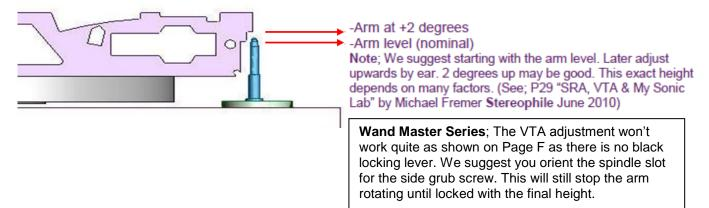
**Step 4**; Position the spindle sideways using protractor Then continue with Page D on the User Guide.
