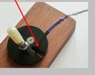
**Step 3**; Position mount using protractor. (Slide or Rotate to get in the correct place).
