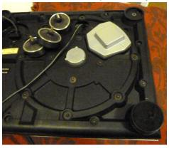
**Step 5**; Remove the three tonearm screws Also the earth wire.
