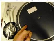
**Step 3**; Remove the feet and rubber base Hint; Leave the screws in place as they are different lengths
