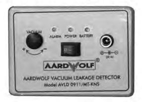
Aardwolf Vacuum Leakage Detector is a battery powered unit consisting of a pressure sensor, an audible warning horn, red warning light and test switch, all controlled by a solid state microchip. It is equipped with a rechargeable Lipo 1-cell battery with a capacity of 3.7V - 2000mAh and the working mode up to 20 operating hours.
