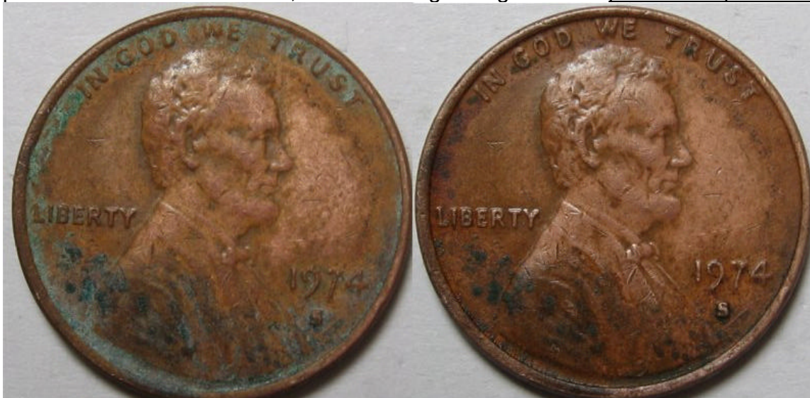
1974-S Lincoln Cent – Previously cleaned before corrosion, light to moderate verdigris on the obverse. Heavy verdigris on the reverse. With a full 24 hour drying period per side and future protection from air and water, the remaining verdigris will be permanently inactive after treatment.
