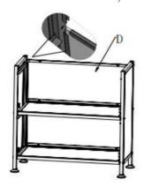
Step 2: Use large screws to connect the left and right lower side panels, (the screws do not need to be tightened);
