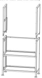
Step 7: Follow steps 2 and 3 to connect the remaining backboards and laminates with large screws;
