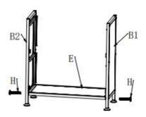
Step 4: Use large screws to connect the left and right lower side panels;
