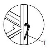
Step 10: Install the cabinet door by pressing the snap button on the cabinet door;
