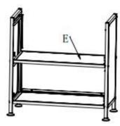
Step 6: Align the left and right upper side panels with the card slots and install them;
