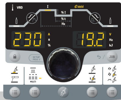
Dual display user interface with rotary knob and push button for fast adjustment of parameters
