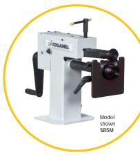
Also available in PLUS version: equipped with 6 standard sets of beading rolls (Nr 3, 4, 5, 22/22, 24 and 26) Ref. SB5M-PLUS
