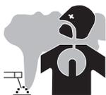
The fumes, gases and dust emitted by welding are harmful to your health. Sufficient ventilation must be provided, an additional air supply may sometimes be necessary. An air-fed mask could be a solution in cases where there is insufficient ventilation. Check that the suction is effective by checking it against safety standards.
