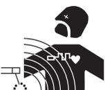
Electric currents passing through any conductor produce localised electric and magnetic fields (EMF). Welding currents produce an electromagnetic field around the welding circuit and welding equipment.
