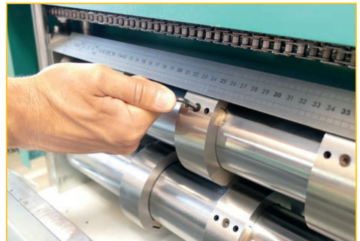
Easy adjustment of slitting blades
