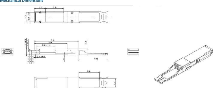
Attention: To minimize MPO connection induced reflections, an MPO receptacle with 8-degree angled end-face is utilized for this product. A male MPO connector with 8-degree end-face should be used with this product as illustrated in Figure below.
