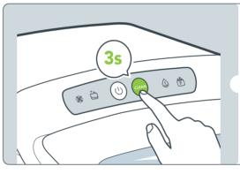
Hold for 3s to start an 8-minute self-cleaning cycle ( stays solid on).
