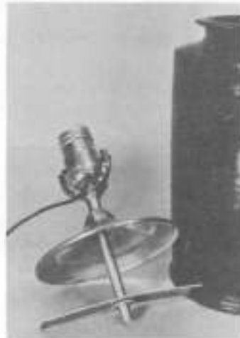
Adapter made with a metal crossbar
