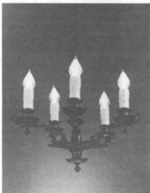
This chandelier is lamped with a bulb (standard-size base) that has fiberglass threads applied—horizontally—to the outside surface. This elongates the hot spot to make it look more flamelike.
