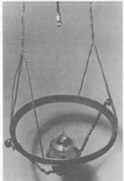
Lamp cord is fastened to chain at right but is still to be fastened to chain at left.
