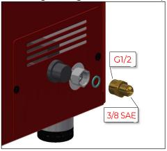
After disconnecting the LPG line, remove the 3/8 SAE connector and its sealing washer. Replace it with the adapter (1) and the new sealing washer (2) provided in the kit.
