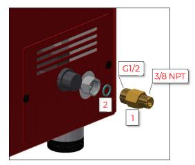
To ensure proper operation, it is essential to replace the orifice with one designed for use with natural gas (NG), as provided in the kit:
